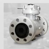
**Trunnion Mounted Ball Valve** 2.1/16" API 5000 - Inconel 625 Body Flanged ends, RTJ type 6B **Engineering: Hyundai Heavy Industries**
