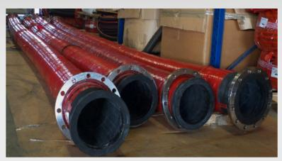
Flexibles hoses for phosphoric acids fitted 8" cam & groove couplings stainless steel 904L
